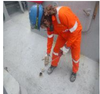
Sounding of Ballast Tank and CH Bilges on Starboard Side
