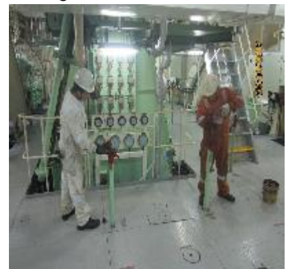
Checking of Tank Sounding in Engine Room
