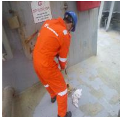
Sounding of Ballast Tank and CH Bilges on Port Side
